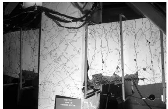
▲ 5.47 Full-scale laboratory test of a beam-column assemblage. A plastic hinge has developed after loading equivalent to a severe quake. Canterbury University.
