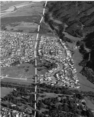
▲ 15.2 A suburb is planned so that an active fault (white dashed line) passes through a green strip. Upper Hutt, New Zealand.
